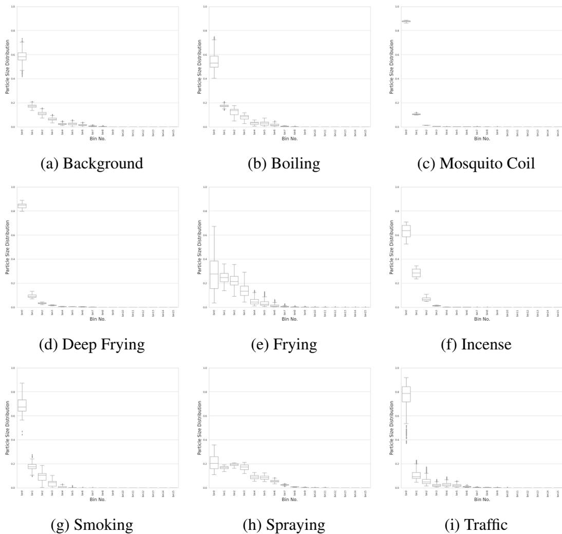
Figure 2.1: Box plots showing the measured individual pollution source PSDs
